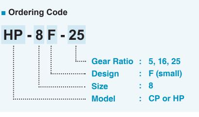
CP - Includes removable input HUB pinion assembly version **HP** - Includes stand alone pinion with precision thru bore
