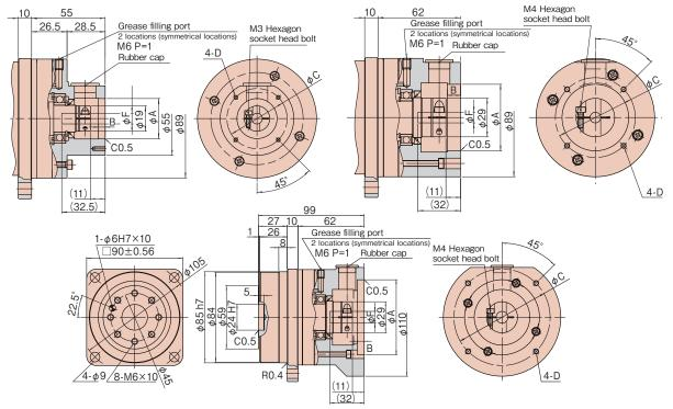
Output shaft shape: J2 (Straight shaft, without key) J6 (Straight shaft, with key, with center tap)
